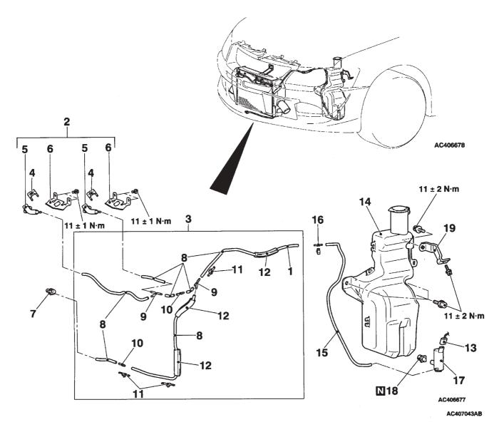
Procedure for removing the water spray nozzle and the hose
