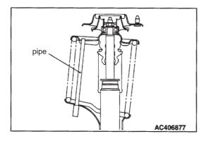
3. Align the holes in the lower spring plate and the upper spring plate of the strut ASSY.
