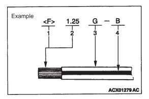
If a cable has two colours, the first colour code indicates the standard colour (the basic colour of the cable coating), and the second colour code indicates the marking colour.
